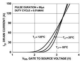
Figure 5. Transfer Characteristics
