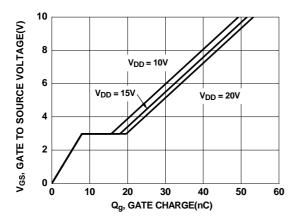
Figure 7. Gate Charge Characteristics
