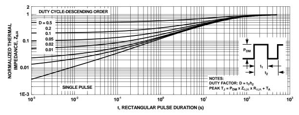
Figure 13. Transient Thermal Response Curve
