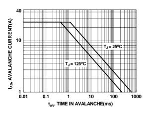
Figure 9. Unclamped Inductive Switching Capability
