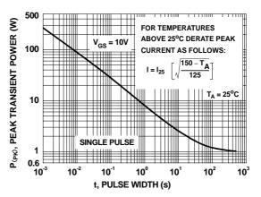
Figure 12. Single Pulse Maximum Power Dissipation
