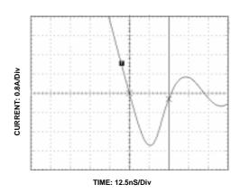
Figure 14. FDMS8670S SyncFET Body Diode reverse recovery characteristics
